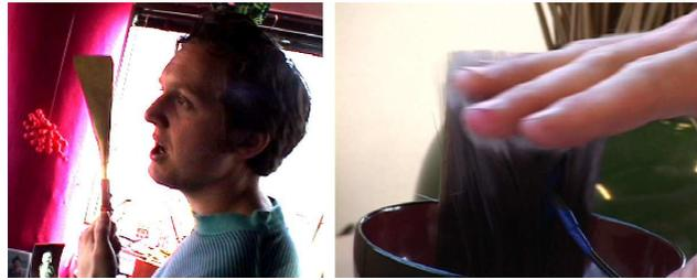
Figure 4: Recording a vocal melody into the system using the wand, and stimulating the piezoelectric sensor directly with soft paintbrush bristles.
