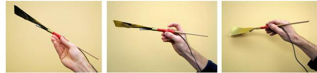
Figure 2: Holding the wand, pressing the record button to capture a sound sample, and scraping the wand against a wall to stimulate the sample.
